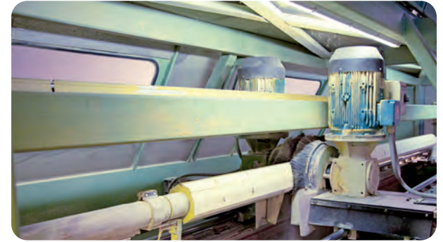
Square and rectangular poles are shaped with a milling cutter.
