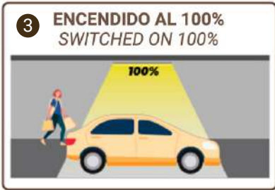
Encendido al 100% tras la detección de movimiento (5s, 90s, 300s, 600s). Switched on at 100% when sensor detects movement (5s, 90s, 300s, 600s).
